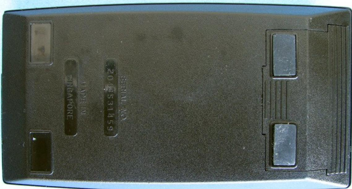
Remove the hatch and you will see two screws (figure 2), remove these.
