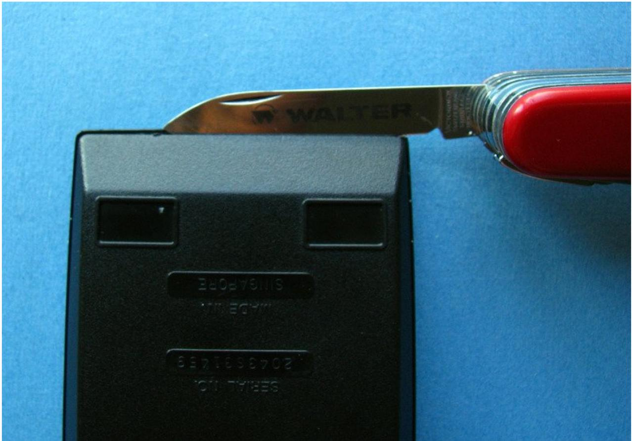
Now that the bottom shell is above the lip of the top shell and while keeping the knife in place to keep the bottom shell out of the top shell recess, give the calculator shells a twist (figure 5). This is a horizontal twist; each shell in the opposite direction of the other. Be gentle as this method does not require force.
